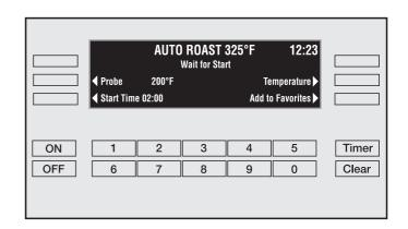
At the end of cooking, when the selected core temperature has been reached, a tone will sound.
